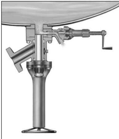
Fig. 2 - Drain Valve Open for Sample
